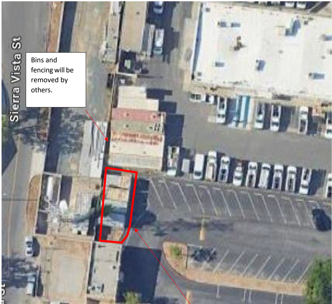
Figure 3: Maintenance yard, demolition scope of work.
